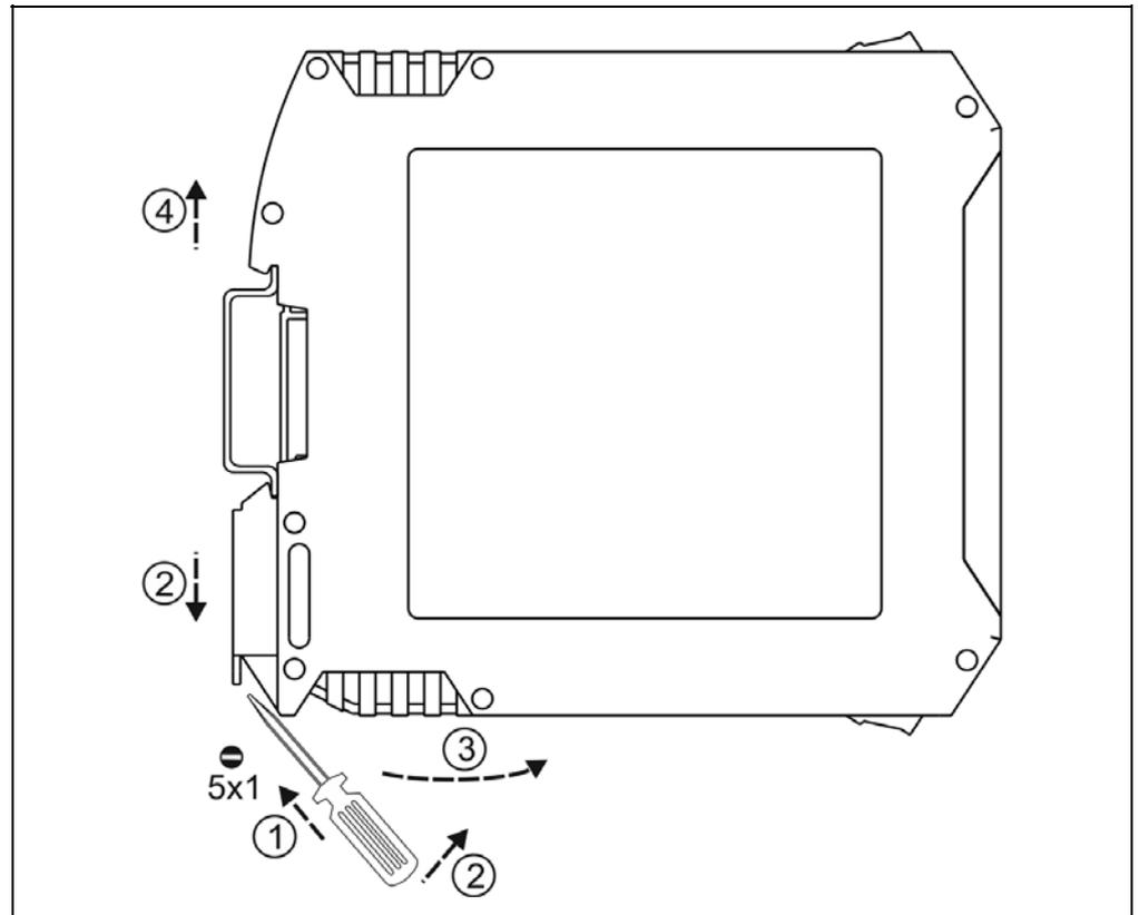
The dismounting procedure needs a screwdriver for slotted screws.
