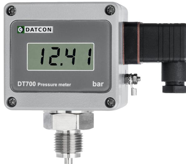
The **DT700 Pressure meters / transmitters** provide a 4-20 mA current proportional to the pressure connected to their input, and they present the measured pressure value on an LCD display.
