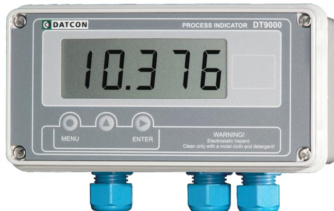
The **DT9000 N, DT9002 N Process Indicators** enable linear process variables to be displayed in engineering units. Two isolated outputs are available with different operating modes for limit signaling or for simple control purposes. Both indicators are looppowered from 4-20 mA signals, dropping less than 2 V at 20 mA.
