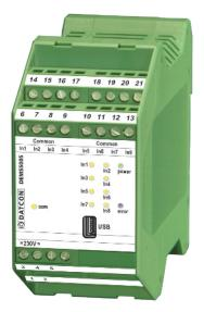
The **DEMS5005 Pulse Collector** has the function to integrate into the system those pulse-output transmitters (volume meters, consumption meters, etc.), which are connected to the inputs of the device. Through the use of this device, it becomes simple to connect various devices to process control systems.
