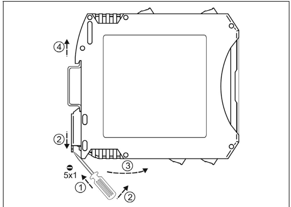
The dismounting procedure needs a screwdriver for slotted screws. Before dismounting disconnect all wires.
