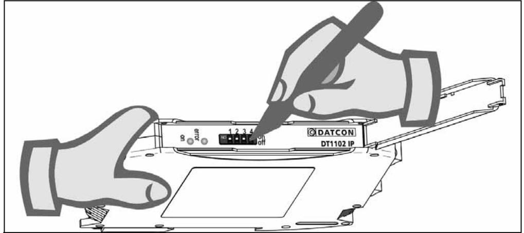
3. Set the configuration switches according to the signal range selection table
