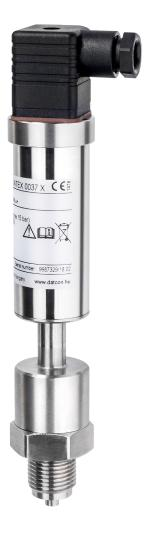
The **DT7200** ...Intrinsically safe pressure transmitters provide a 4-20 mA current signal in proportional to the pressure connected to their input. The transmitters are intrinsically safe devices, and they can be operated in a potentially explosive environment falling into the category Zone 0 and Zone 1.
